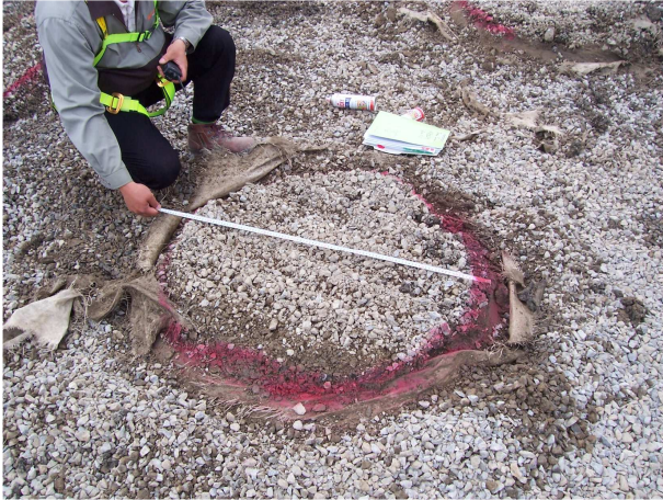
Figure 2. Measurement of the diameter of a stone column close to ground surface.
