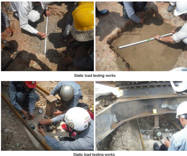
Figure 3. Load test on a single stone column.
