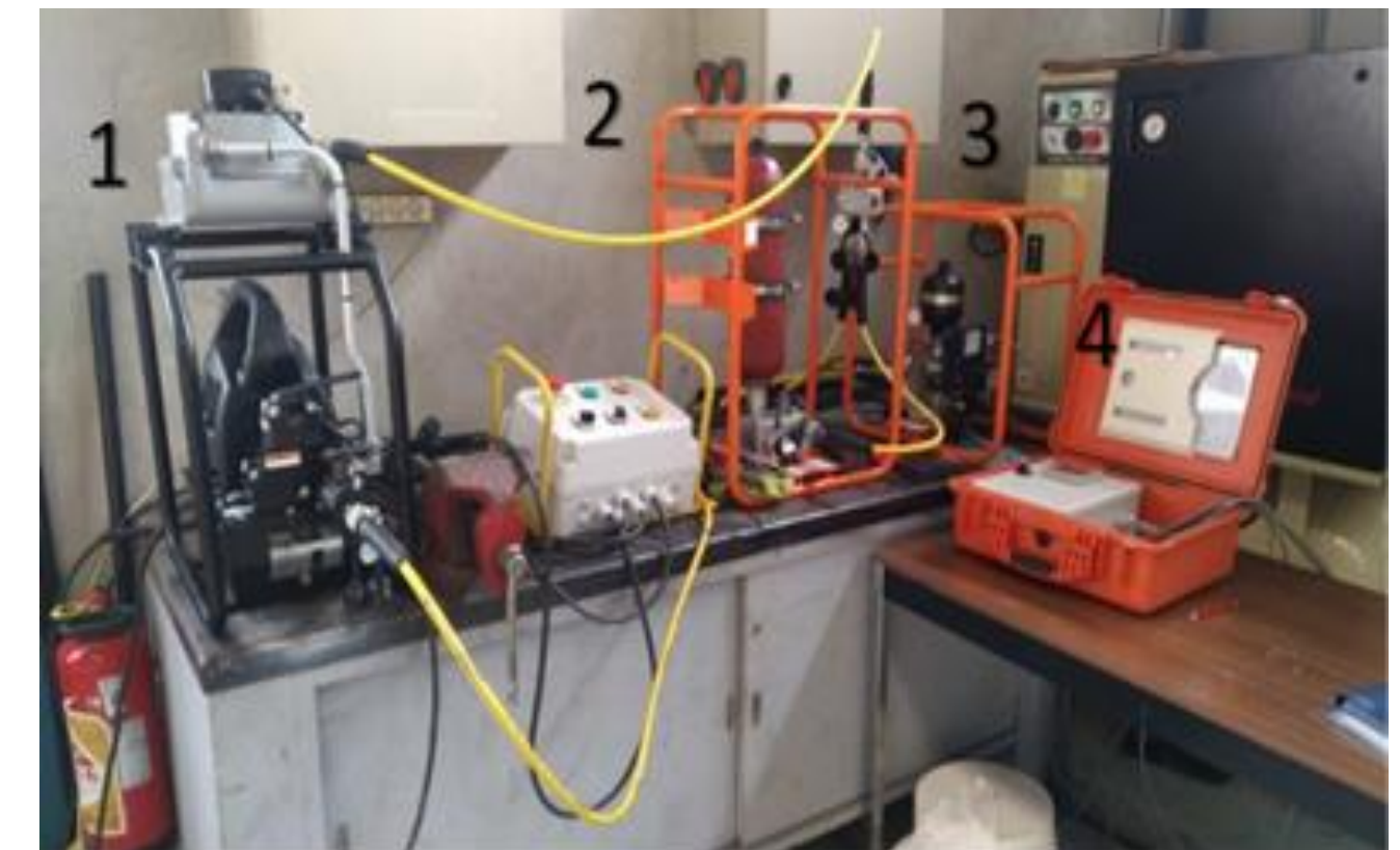
Dynamic nail pull-out device
