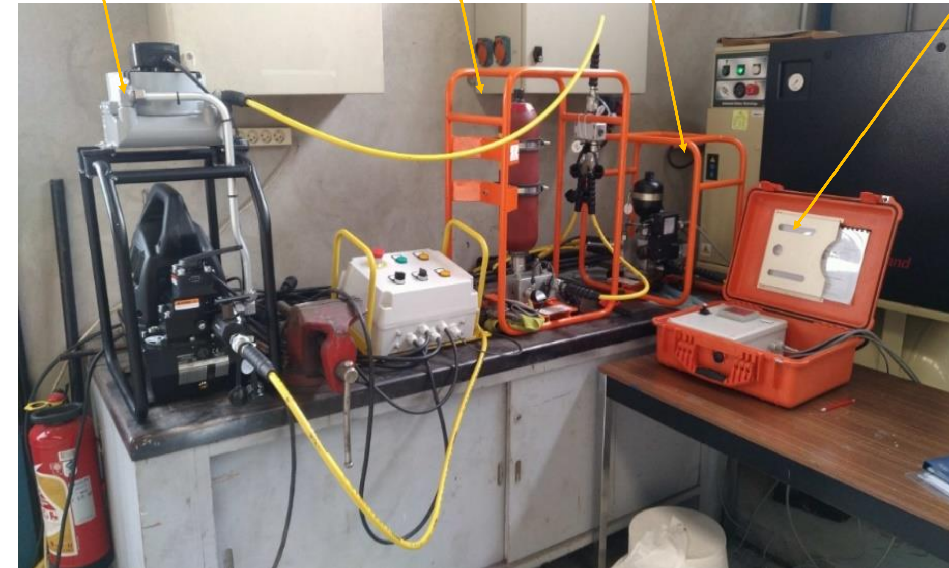
The dynamic pull-out device
